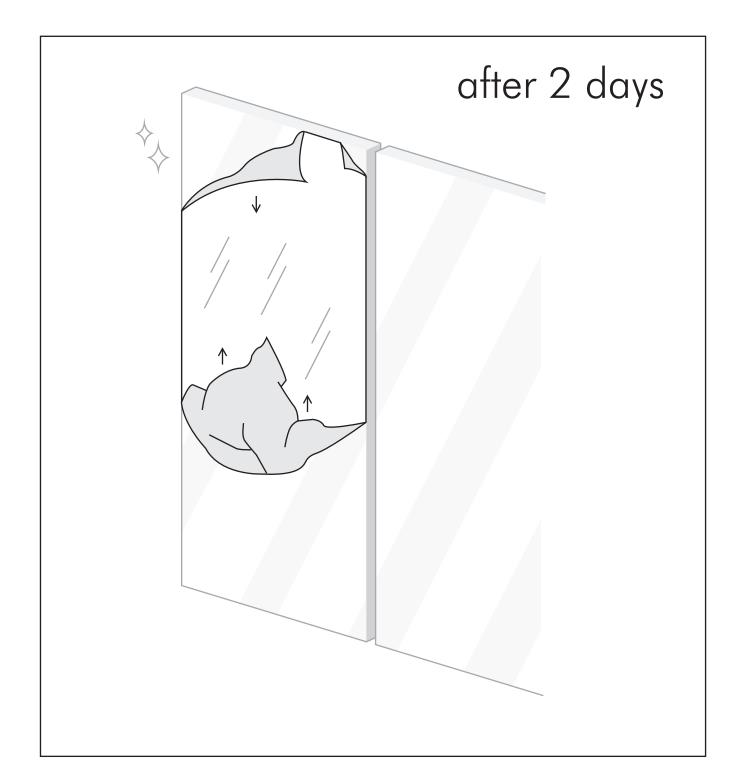
Remove protection film after 2 days of panel application. Slowly pull the film towards the center of the panel.
