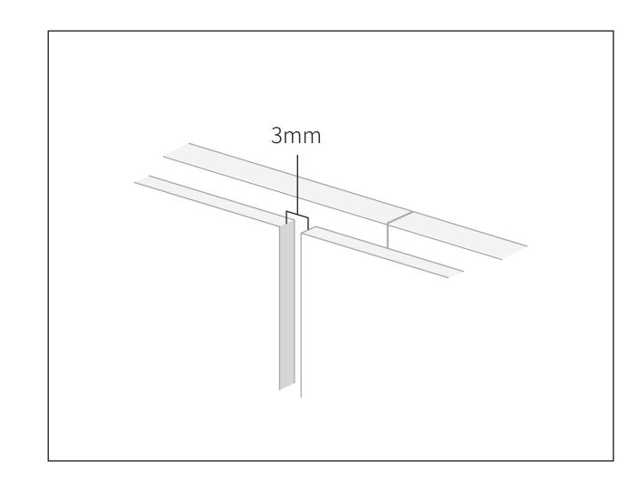
Joint of substrate and joint of wall panel should be laid out in different position. If wall panels are applied without gap in between, they could be delaminated by expansion. The gap should be at least 3mm wide.
