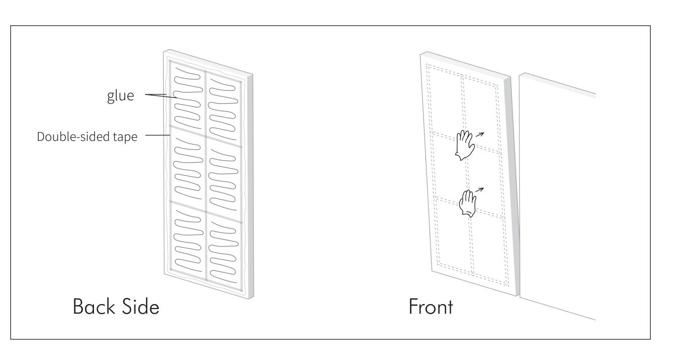
During application, make sure the center of the panel is completely applied onto the substrate.
