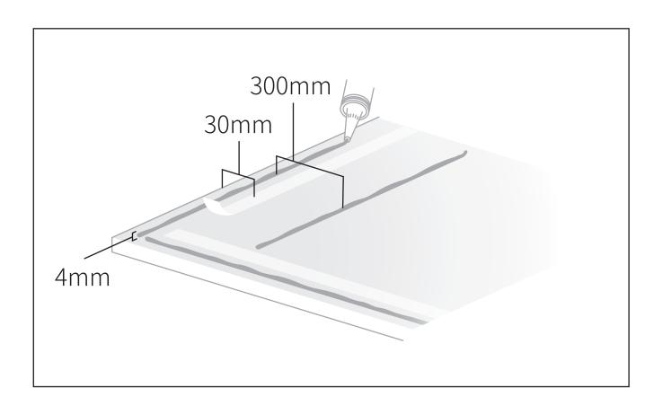
Do not forget to apply the adhesive on the edges. Otherwise, it could be delaminated. The adhesive should be applied 4mm by height; one column of adhesive should be 300mm away from the next column. After the adhesive application, the panel should be applied onto substrate under 10 minutes.
