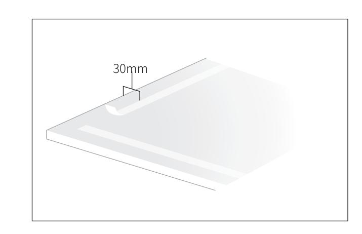
Apply double-sided tape 30mm away from edge of the panel. This gives a temporary fix until the adhesive dries completely.
