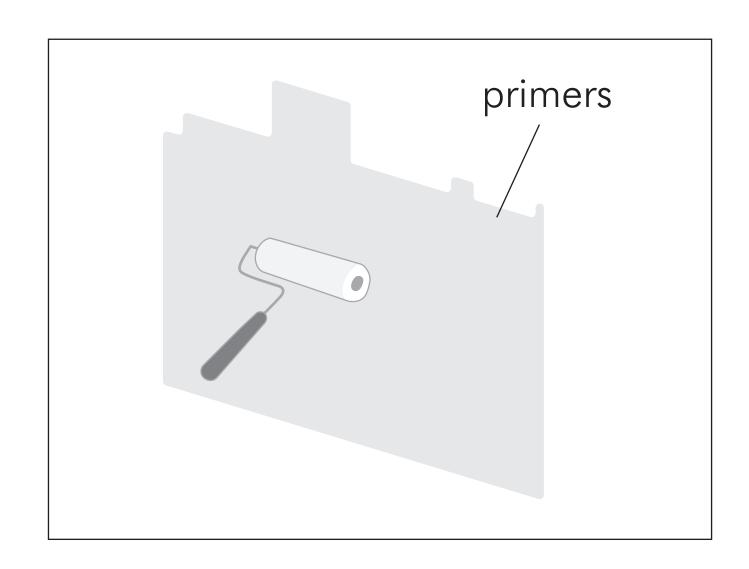
Apply primer on substrate in advance if substrate is concrete, plywood or gypsum board. Ensure that substrate is flat and cleansed with cleaning agent.
