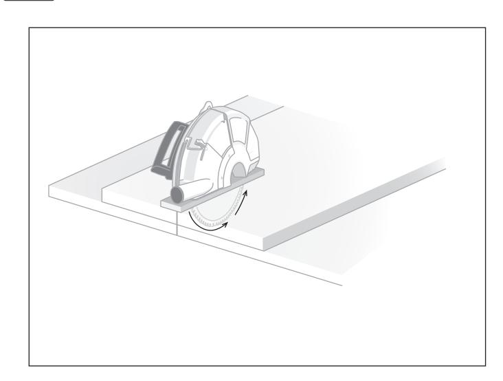
Use splint in order to keep the cutting edge clean. The cutter should start cutting from the top face of the panel and cut through completely.
